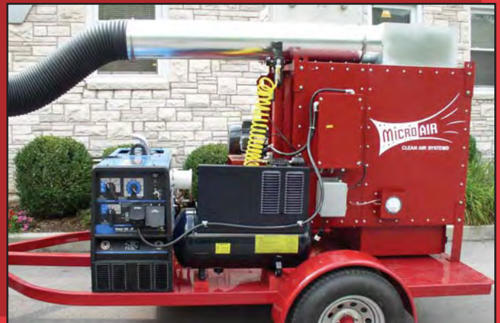
Trailer mounted RP4 collects cement dust
