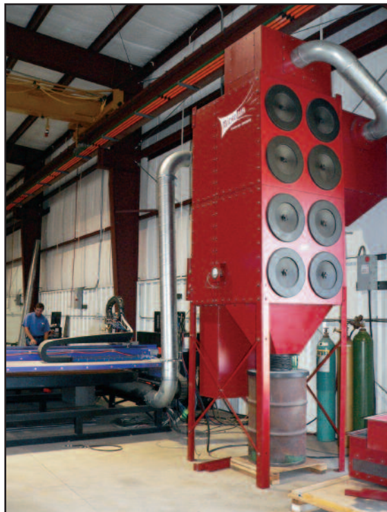
RP8 with Spark Arrestor collects smoke/fumes from plasma table
