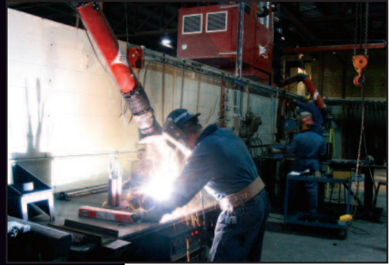
Source Capture of Weld Smoke and Fumes
